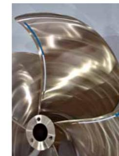
"The prop uses different height strips to alter the pitch and find the optimum setup."
