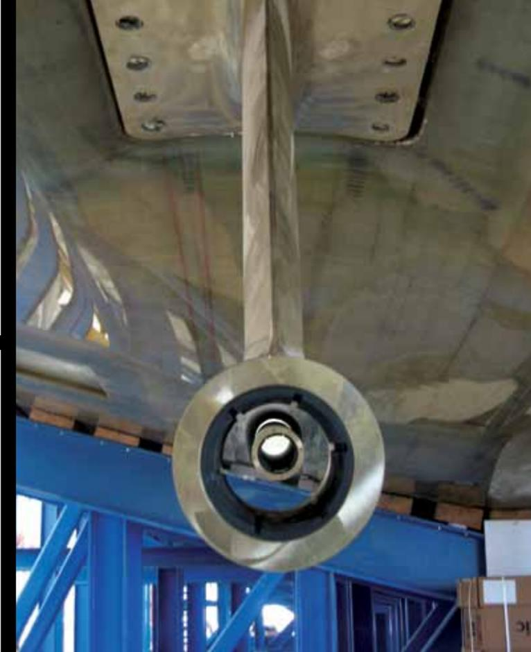
micrometers, which can then be adjusted up and down or side-to-side and measurable in thousandths of an inch. "When that laser beam shoots up to a target plate on the transmission's coupling and it hits the bull's eye, we know we've got it right." Marsh added.
